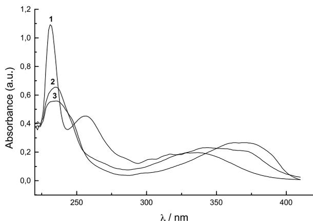
**Figure 3.** UV–visible absorption spectra for the compounds **1–3** in  $\text{CH}_2\text{Cl}_2$  at room temperature and  $[c] = 10^{-5} \text{ M}$ .
