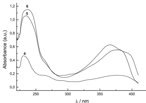
**Figure 5.** UV–visible absorption spectra for the compounds **4–6** in  $\text{CH}_2\text{Cl}_2$  at room temperature and  $[c] = 10^{-5} \text{ M}$ .
