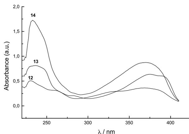
Fig. 9. UV-visible absorption spectra for the compounds **12–14** in  $\text{CH}_2\text{Cl}_2$  at room temperature and  $[c]=10^{-5}$  M.
