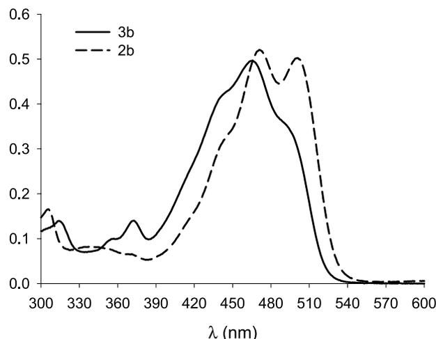
Figure 2. Electronic absorption spectra of **2b** and **3b** ( $10^{-5}$  M in  $\text{CH}_2\text{Cl}_2$ ).
