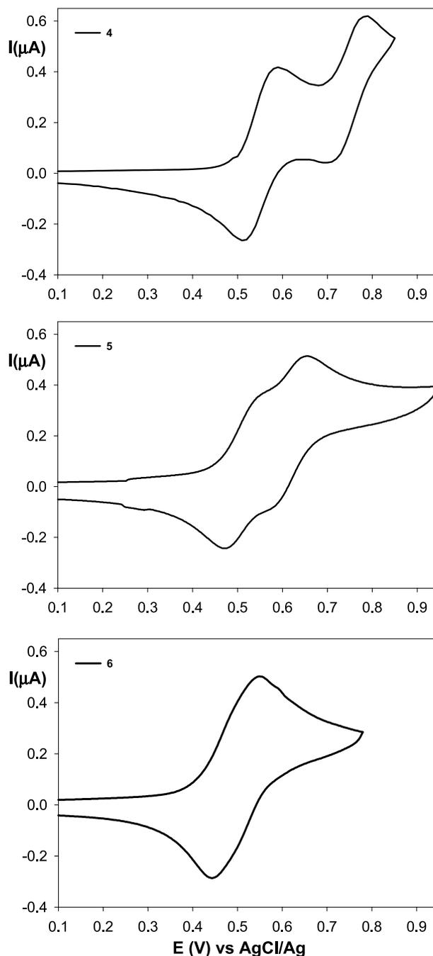
**Figure 5.** CV of oligomers **4–6** ( $10^{-4}$  mol L<sup>-1</sup> in 0.1 M Bu<sub>4</sub>NPF<sub>6</sub>/CH<sub>2</sub>Cl<sub>2</sub>), scan rate 100 mV s<sup>-1</sup>.
