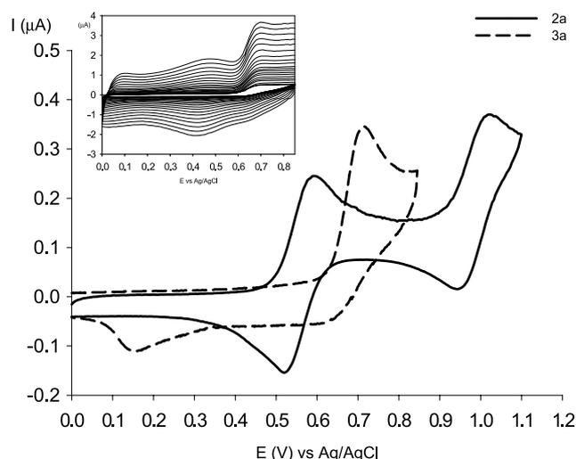
Figure 4. CV of oligomers **2a** and **3a** (saturated solution in 0.1 M  $\text{Bu}_4\text{NPF}_6/\text{CH}_2\text{Cl}_2$ , scan rate  $100 \text{ mV s}^{-1}$ ; insert) electropolymerisation of **3a** by application of successive potential scans.
