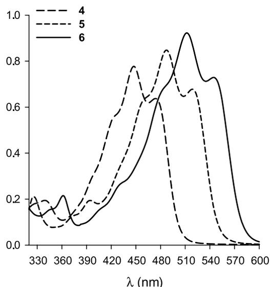
Figure 3. Electronic absorption spectra of **4**, **5** and **6** ( $10^{-5}$  M in  $\text{CH}_2\text{Cl}_2$ ).
